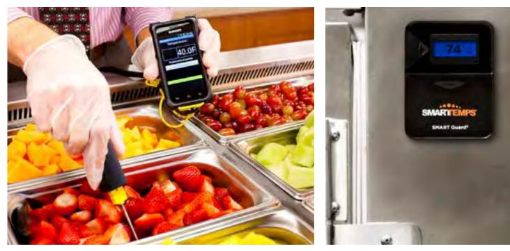
SMART TEMPS The Mishawaka company's technology monitors the temperature of things that need to be cold or hot, and automatically sends out email, text or phone alerts if a sensor senses that something isn't the way it should be.
